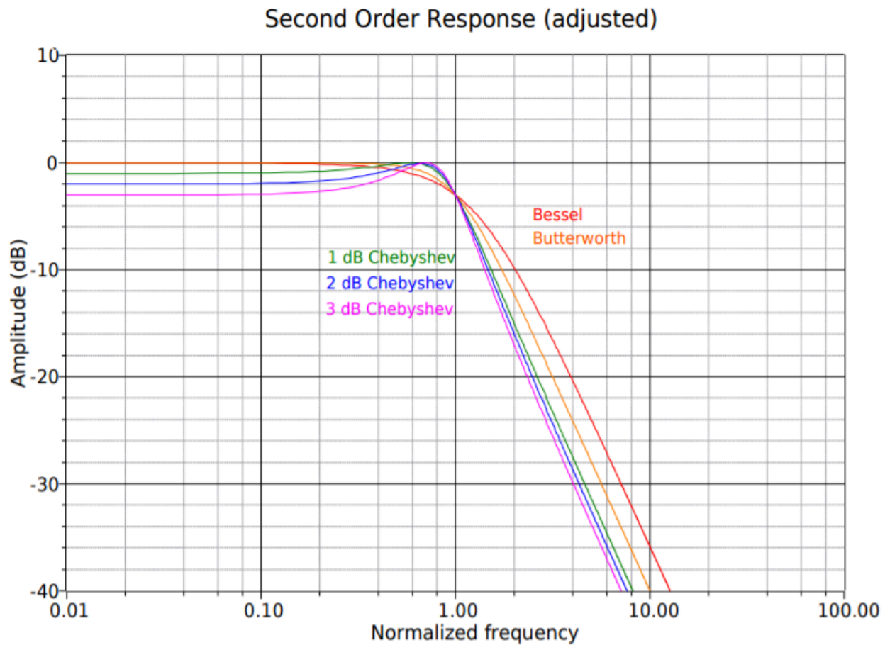
Figure 11.5.1 ♦ : A comparison of the major filter alignments: second order response (adjusted).
