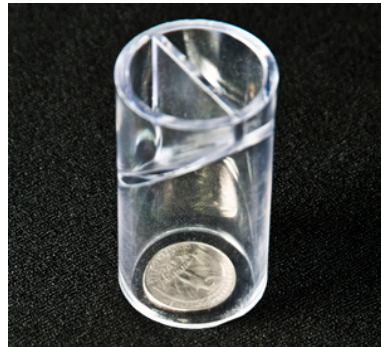
Figure 3.18 – This is a small parts tester (or choke tube). If an item/toy fits inside, it's a choking hazard.
