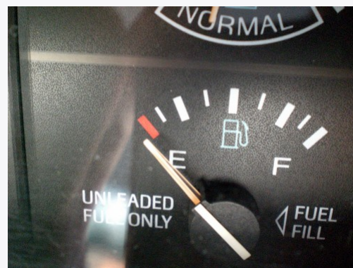
Figure 4. Because the gas expands more than the gas tank with increasing temperature, you can't drive as many miles on “empty” in the summer as you can in the winter. (credit: Hector Alejandro, Flickr)
