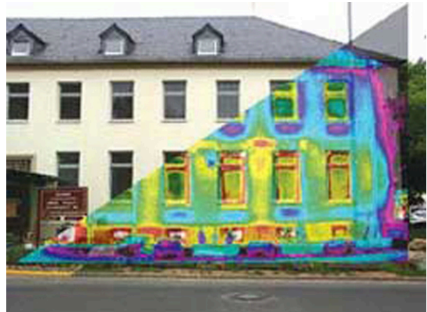
Figure 5. A thermograph of part of a building shows temperature variations, indicating where heat transfer to the outside is most severe. Windows are a major region of heat transfer to the outside of homes. (credit: U.S. Army)
