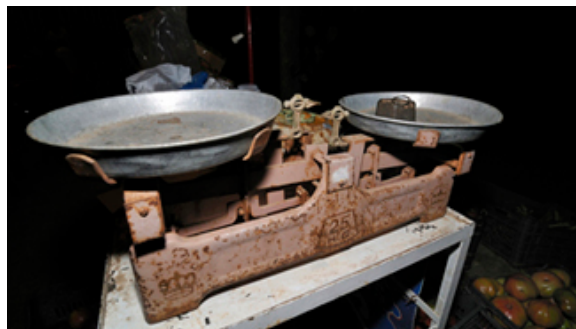
Figure 1. A double-pan mechanical balance is used to compare different masses. Usually an object with unknown mass is placed in one pan and objects of known mass are placed in the other pan. When the bar that connects the two pans is horizontal, then the masses in both pans are equal. The “known masses” are typically metal cylinders of standard mass such as 1 gram, 10 grams, and 100 grams. (credit: Serge Melki)
