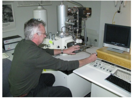
Figure 7. An electron microscope has the capability to image individual atoms on a material. The microscope uses vacuum technology, sophisticated detectors and state of the art image processing software. (credit: Dave Pape)
