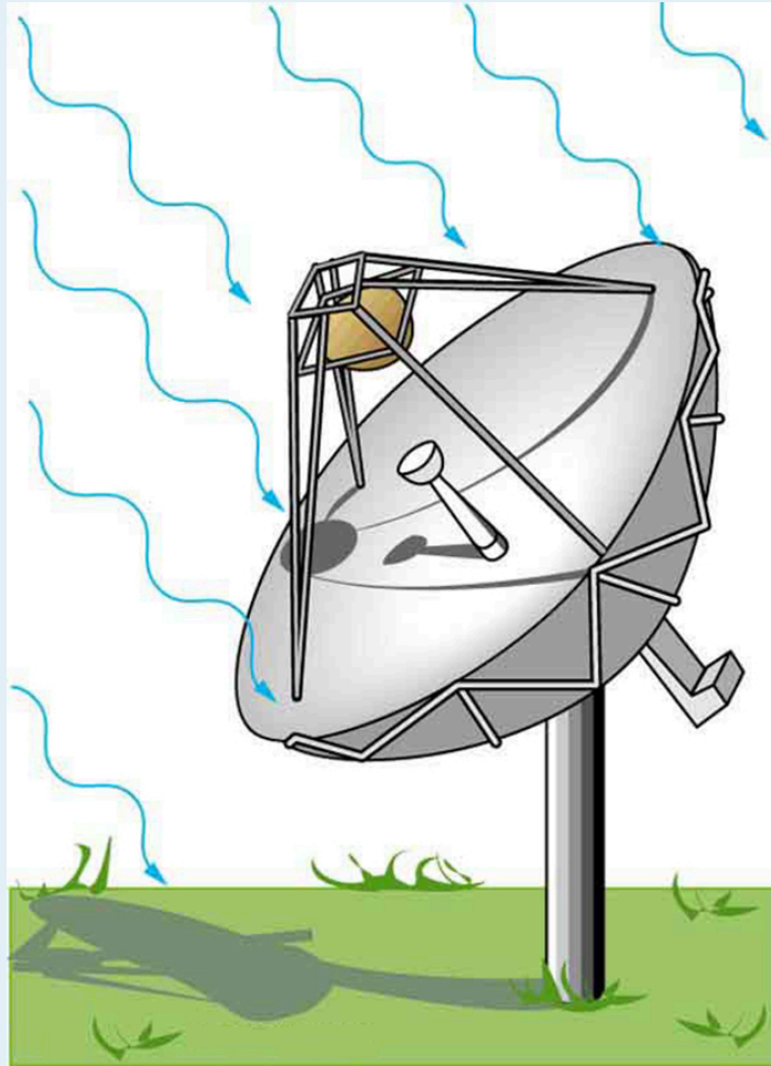
Figure 2. Satellite dishes receive TV signals sent from orbit. Although the signals are quite weak, the receiver can detect them by being tuned to resonate at their frequency.
