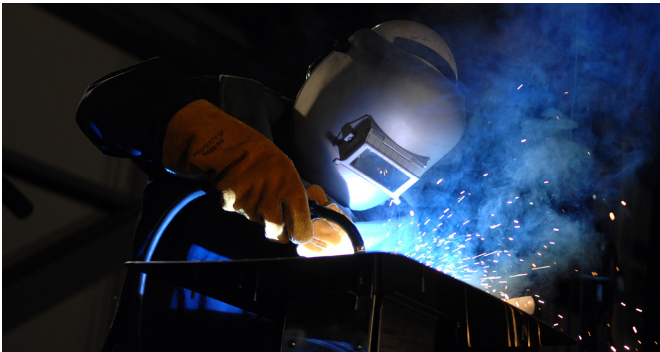
Figure 1. The welder's gloves and helmet protect him from the electric arc that transfers enough thermal energy to melt the rod, spray sparks, and burn the retina of an unprotected eye. The thermal energy can be felt on exposed skin a few meters away, and its light can be seen for kilometers. (credit: Kevin S. O'Brien/U.S. Navy)
