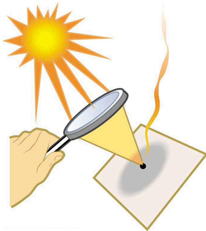
Figure 2. Sunlight focused by a converging magnifying glass can burn paper. Light rays from the sun are nearly parallel and cross at the focal point of the lens. The more powerful the lens, the closer to the lens the rays will cross.
