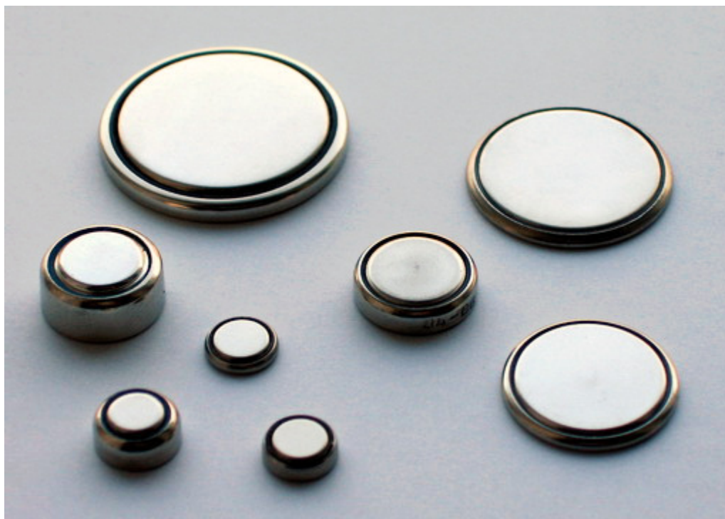
Figure 16.3 Button Batteries. Button batteries like those seen here can be used for a variety of portable electronics, from watches and hearing aids to handheld gaming devices.
