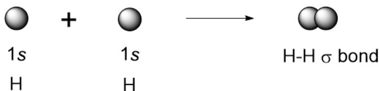
Figure 10.6. A diagram showing the overlap of s orbitals of two hydrogen atoms to form H_2 .
