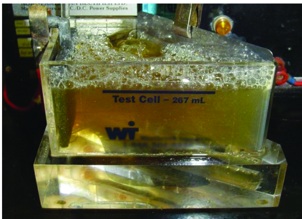
Figure 16.6 “Electroplating.” Electroplating on a test cell. Credit: courtesy of Fstep, http://commons.wikimedia.org/wiki/File:Hullcell.jpg .
