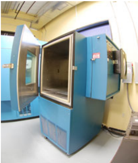
Product Testing: This is a photo of a temperature and humidity chamber used to simulate transport, warehouse environments, and shelf life conditions of a packaged product.
