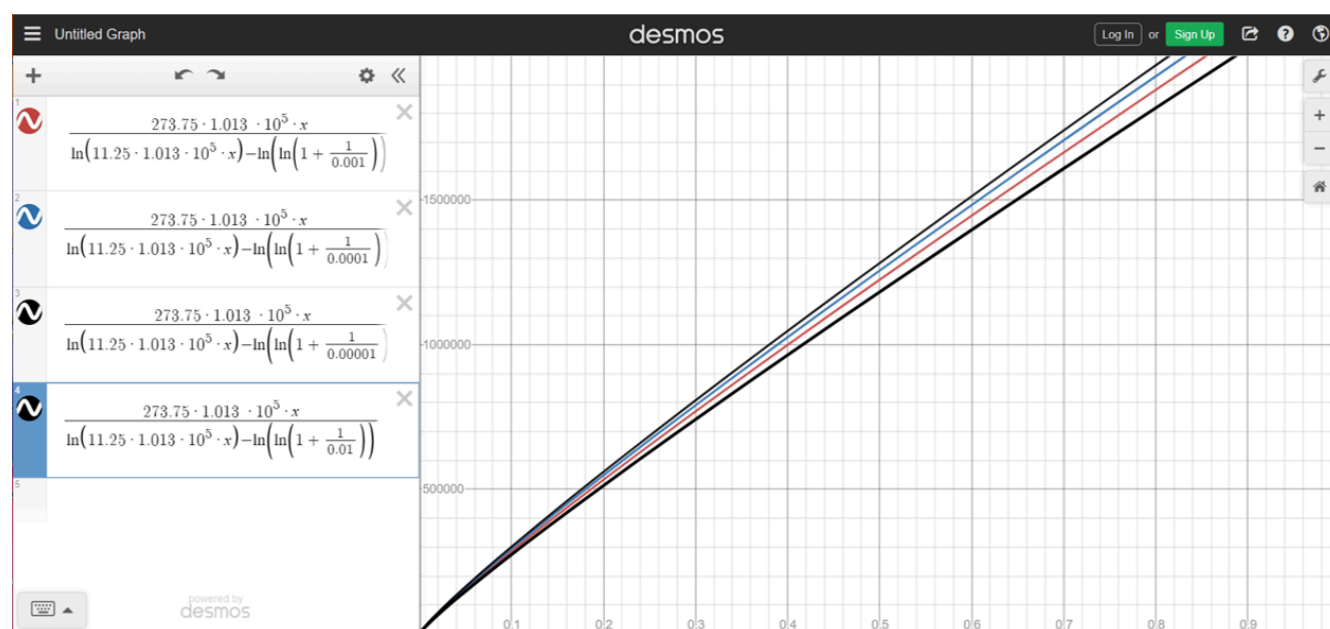
Plots of Paschen's Law for air at atmospheric pressure and values of the secondary emission coefficient equal to 0.01, 0.001, 0.0001, 0.00001.
