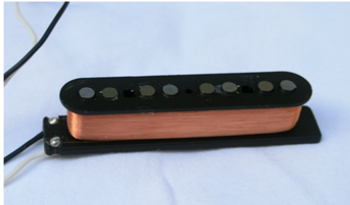
Figure 6.4.5: Electric bass pickup (cover removed).
